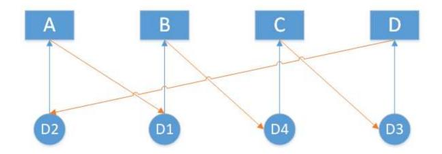
Process A is holding D2 device and has requested for D1. D1 is held by process B and process B has requested for D4, D4 is held by process C and process C has requested for D3. D3 is currently held by process D and process D has requested for D2 that is held by process A. So, there is a deadlock.
